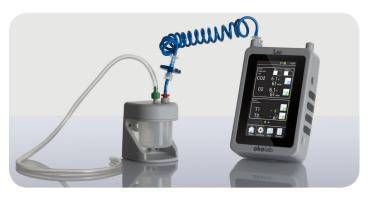
The Moisture Trap (included with LEO) is used when the measured gas is wet, in order to retain water molecules.
