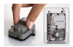
Other (external) sensor modules can be connected to LEO's connection ports.
